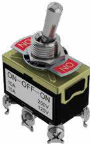
4494 Interruptor uso industrial DPDT ON-OFF-ON 15A 125V / 10A 250V~
